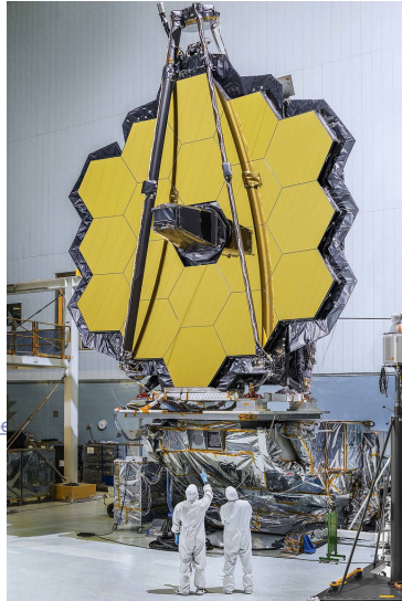
Fig. 40 The primary mirror of NASA's James Webb Space Telescope, consisting of 18 hexagonal mirrors, looks like a giant puzzle piece standing in the massive clean room of NASA's Goddard Space Flight Center in Greenbelt, Maryland.
