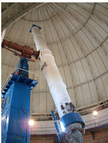
Fig. 24 Yerkes Observatory 40 inch Refractor Telescope ( It is the largest refracting telescope used for astronomical research.) Williams Bay, Wisconsin, US
