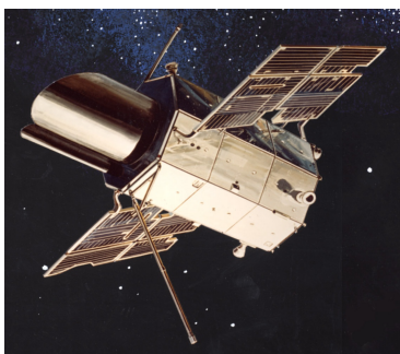
Fig. 35 The Orbiting Astronomical Observatory (OAO) satellites were a series of four American space observatories launched by NASA between 1966 and 1972, which provided the first high-quality observations of many objects in ultraviolet light.
