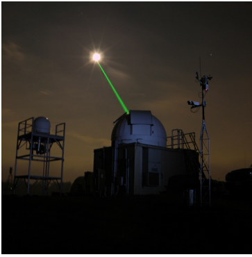
Fig. 3 Goddard's Laser Ranging Facility directing a laser (green beam)
