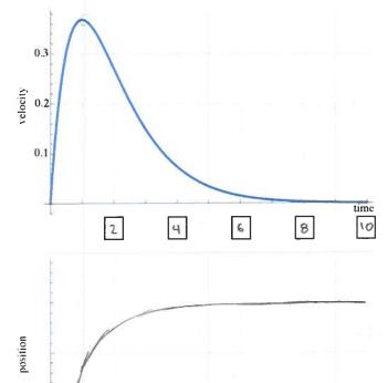
Here are 3 plots. In the middle, we have the velocity of an object as measured by our Velocity-Measure-O-Matic™. Through some fancy curve fitting, we found it followed a very simple function of time:
