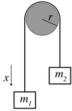
4. In the figure are two masses,  $m_1$  and  $m_2$ , connected via a massless rope around a *massive* pulley. The pulley has a mass of  $M$  and radius  $r$ .
