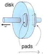
4. A disk brake works by squeezing two pads against a rotating disk. A large kinetic friction force is created between the pads and the disk, which reduces the angular velocity of the disk. Use the following parameters to answer the questions below:
